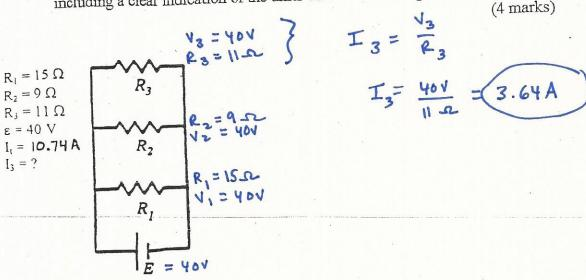
15. In the circuit diagram given below, determine the value of I<sub>t</sub>, the current supplied by the source. Your answer must include the formulas used and all of the calculations, including a clear indication of the units of measure throughout the calculations.
