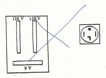
20. In more modern houses, the double outlets above the kitchen counter have two independent circuits. Give the main reason for this set-up. (3 marks)
