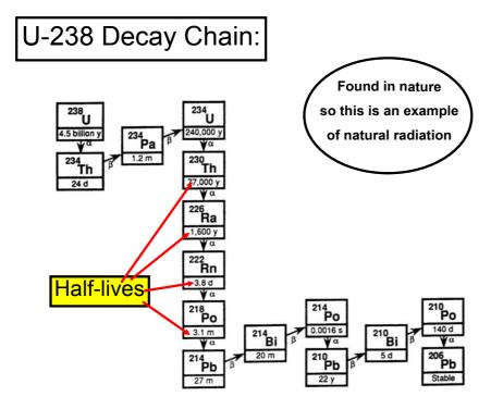
Half-life: for a radioactive isotope, it is the amount of time that it takes for half of the atoms in a sample to decay (e.g. by α- or β-decay) into a different element.
