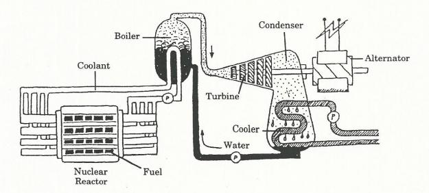
A nuclear power station operates on the same principle as a conventional thermal power station, only the oil or coal is replaced by nuclear fuel.
