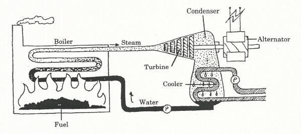
A conventional thermal power station uses energy from a fossil fuel (heating oil or coal). The steam produced is used to drive a turbine, which in turn drives a generator.
