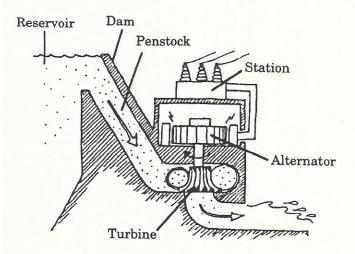
A hydroelectric power station converts water's gravitational potential energy into electrical energy.
