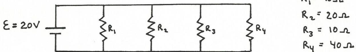
2. Do a complete analysis of the following circuit after drawing the corresponding simple equivalent circuit.
