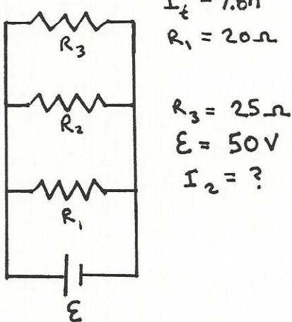
$$\begin{aligned}I_t &= 7.8A \\R_1 &= 20\Omega \\R_3 &= 25\Omega \\\epsilon &= 50V \\I_2 &=?\end{aligned}$$
