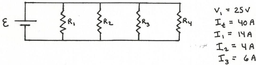
3. In the circuit diagram below, determine the value of  $I_t$ , the current supplied by the source. Your answer must indicate the formulas used and must include all calculations, including a clear indication of the units of measure throughout the calculations.
