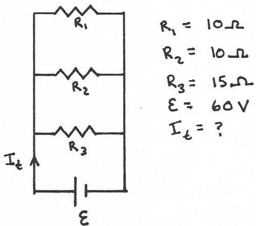
$$\begin{aligned}R_1 &= 10\Omega \\R_2 &= 10\Omega \\R_3 &= 15\Omega \\\epsilon &= 60V \\I_t &=?\end{aligned}$$
